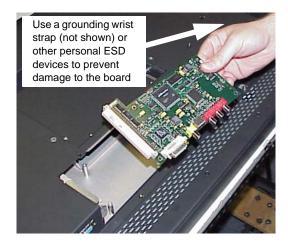
6. Carefully slide the right side of the board into the slot on the right side of the opening.
